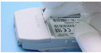
The SRT-6 opening tool is also very helpful, when opening the Antenna.
