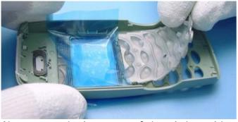
Also, protect the inner part of the window with a foil. The Keymat is loose inside the cover.
