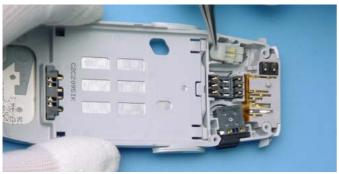
The Vibra Motor with its rubber housing is pressed into the D-Cover.
