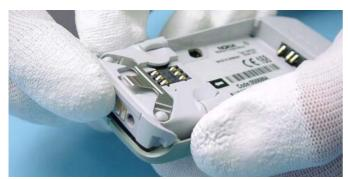
Take care that your workbench is always clean and protect the Window with a foil against dust and scratches. Release the A-Cover from the bottom side of the unit.
