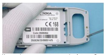
You need some power to press the Antenna Pogo Pins from the D-Cover.
