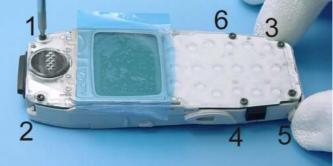
Open the six screws in the predefined order with a Torx 6 driver. When re-assembling, the reverse order has to be taken with a torque of 30 Ncm.
