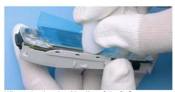
When releasing the side clips of the D-Cover you can use plastic tweezers or the opening tool from 5510 (SRT-6, 0770431), as shown in the picture.
