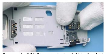
Remove the SIM Connector by hand. Note the right direction, when replacing the SIM connector. It only fits in one direction.
