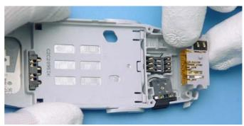
No special tools are needed to remove the System Connector. Note that the Microphone cannot be changed separately (like in other products), because it is one unit with the System Connector.
